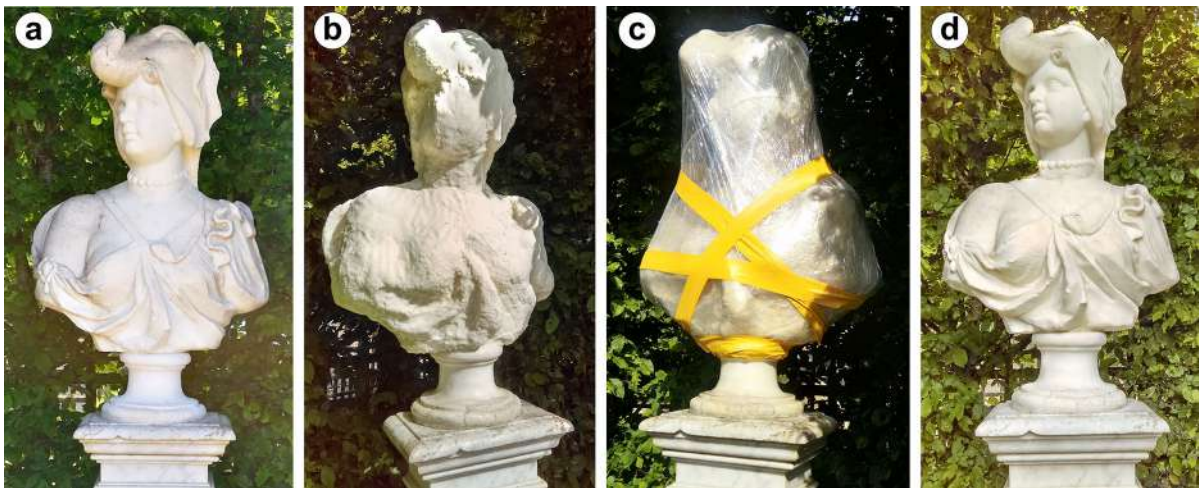
Fig. 4 Phases of bust consolidation: a before treatment; b after poultice application; c after wrapping with a plastic film; d after treatment
