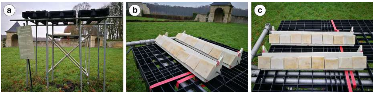
Fig. 2 Specimen exposure in the Park of the Versailles Palace: a height from the ground; b 45° inclination with respect to the horizontal; c distancing among the specimens
