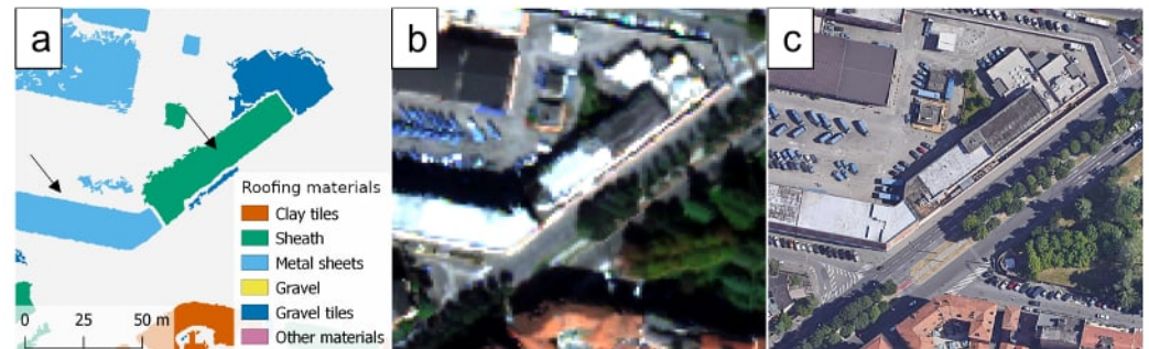
Figure 11. (a) Classification map detail, where the two blocks indicated by the arrow are both covered by sheath; (b) corresponding WV3 image used for the classification; (c) another high-resolution image of the same area (from Google Earth [52]).
