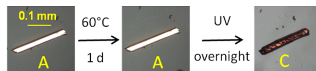
Figure 2. Cross-polarized HSM pictures showing single crystals of [1H]Br form A before and after thermal treatment and after UV irradiation.
