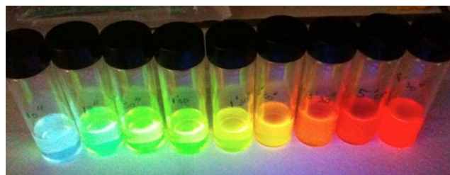
Fig. 2 Photograph of chloroform solutions of CdSe-ZnS QDs of different size (smaller to larger from left to right) under UV excitation.
