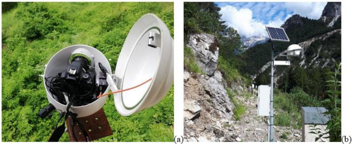
Figure 2. Photographic system survey. (a) Hardware system components; (b) Photographic system set up in Perarolo, on the opposite side of the landslide.
