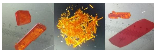
Figure 2. Single crystals of compounds 1 (left), 2 (middle) and 3 solv. (right) obtained by recrystallization from solution of the mechanochemical synthesis products (see Experimental).
