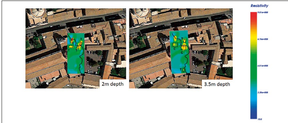
Fig. 7 – Electrical Resistivity Tomography (ERT) resistivity depth slices.
