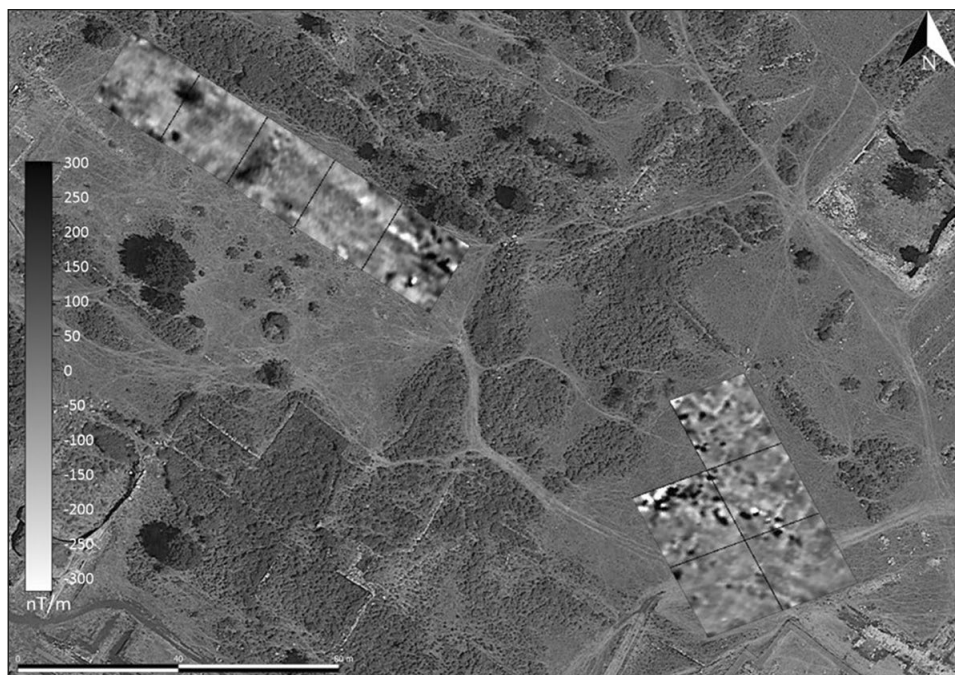
Fig. 4 – Contour map of the gradient of the vertical component Z of the earth magnetic field. Range -300 -+300 nT/m.
