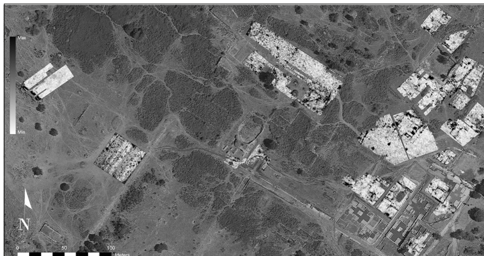
Fig. 2 – GPR time slices at the estimated depth of 0.90 m for all investigated areas.
