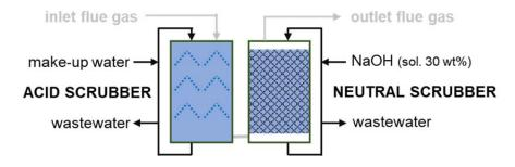
Figure 1: Reference scheme for the wet scrubbing system.
