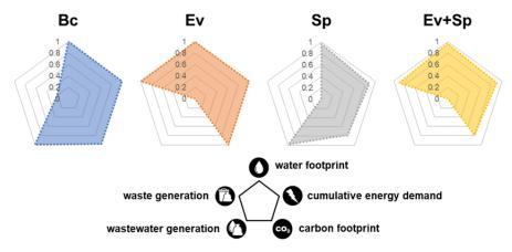
Figure 3: Normalised impact indicators for the alternatives under study. Case 1 of flue gas composition.
