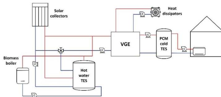
**Figure 1.** View of the building. **Figure 2.** Layout of the ejector-based cooling system.
