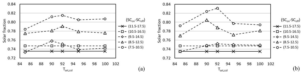
**Figure 3.** Solar fraction achieved with the proposed logic as a function of control settings. Data reported for  $T_{set, TES} = 90^\circ\text{C}$  (a) and  $T_{set, TES} = 95^\circ\text{C}$  (b).
