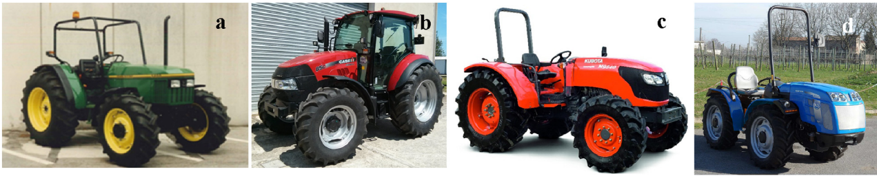
Fig. 1. Tractor ROPSs; (a) four post frame, (b) cab, (c) rear two post, (d) front foldable two post.
