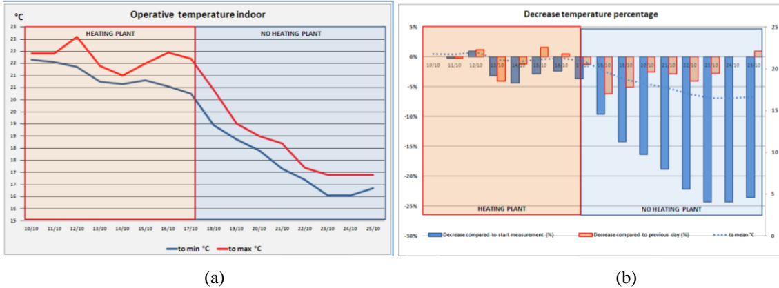
FIGURE 6 (a) Indoor minimum and maximum operative temperature with HVAC on (10-16 October) and off (17-25 October): (b) Graphics 8 Decrease temperature percentage
