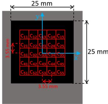
Fig. 5. Sensing area dimensions with taxel distribution.
