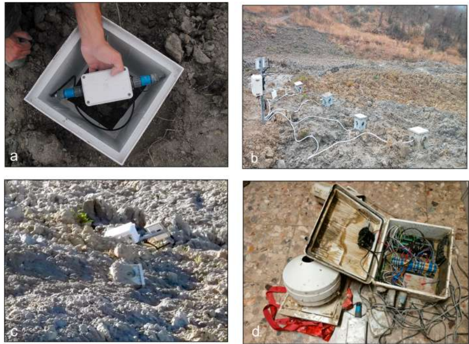
Figure 7. Photographs of the Montevecchio monitoring system. (a) Geophone amplifiers inserted in a plastic box; (b) continuous monitoring system installed in the main track of the earthflow channel. (c, d) Equipment damaged by a reactivation of the earthflow.
