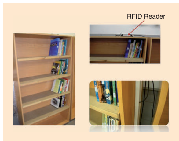
Figure 45. The prototype library cabinet with four shelves. The shelf antennas are fed on the side with coaxial cables running from the reader's ports or the multiplexer. Books (equipped with RFID tags) reside on top of the shelf antennas.
