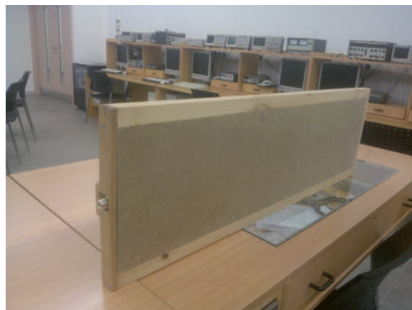
Figure 46. The shelf antenna with an N-type connector on the side.
