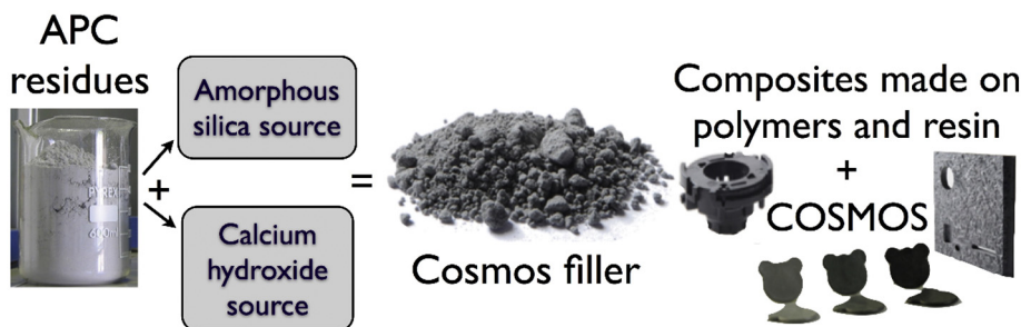
Fig. 3. Schema of the COSMOS process (the main materials used for stabilization are amorphous silica and calcium hydroxide). This Figure also shows some composites materials that have been produced by using COSMOS.
