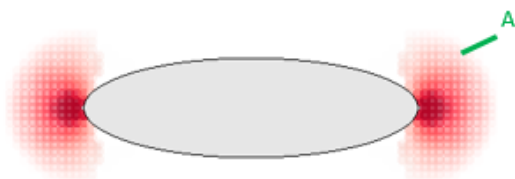
a) Isolated crack full-space
