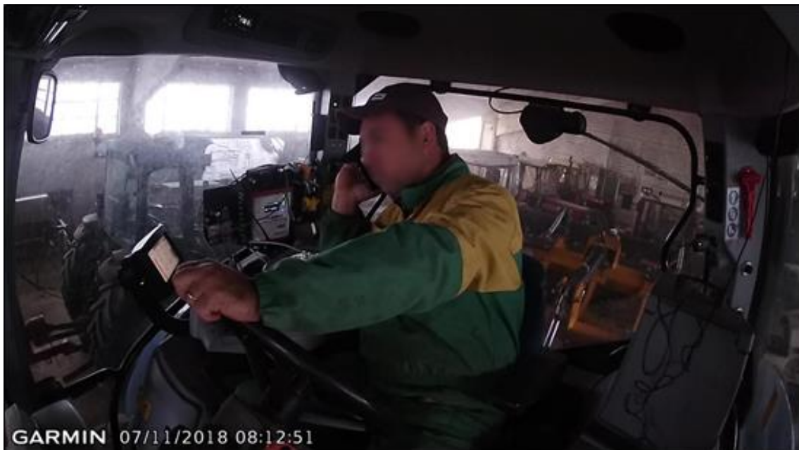
Fig. 9: Frame of a video recorded with the dash cam where the idling stop was caused by a phone call.
