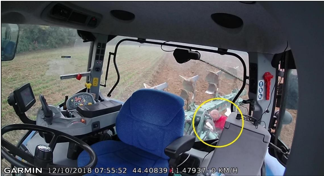
Fig. 5: Frame of a video recorded with the dash cam where the idling stop was caused by an adjustment of the skim coulters of the plough.
