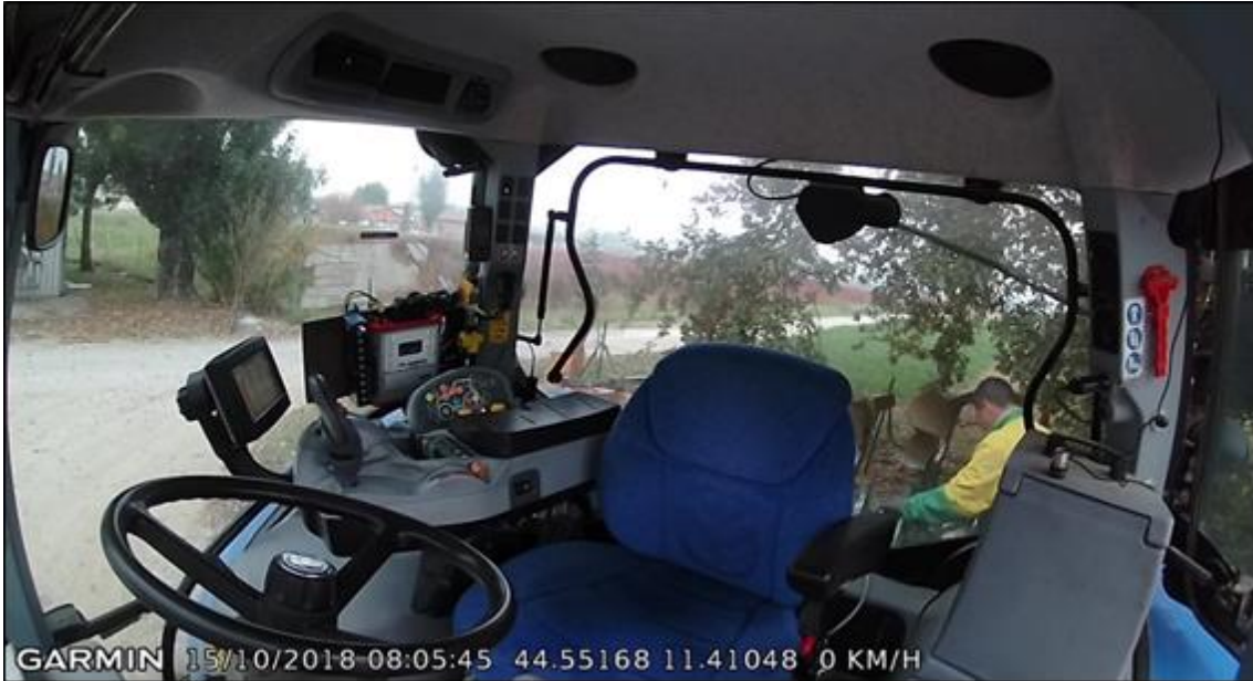
Fig. 4: Frame of a video recorded with the dash cam where the idling stop was caused by the hitching of a plough.
