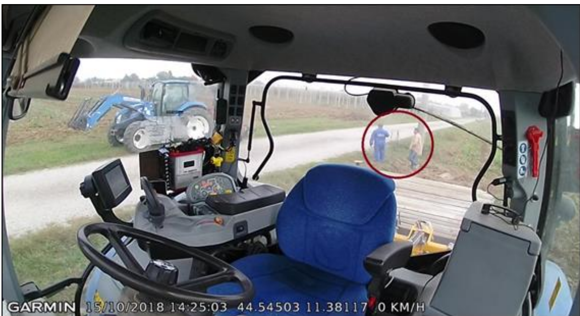
Fig. 6: Frame of a video recorded with the dash cam where the idling stop was caused by a talk between drivers.
