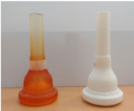
Fig. 5 Additively manufactured trombone mouthpieces: the SLA version in orange on the left and the FDM one in white on the right
