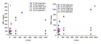
**Figure 8.** Static binding capacity at various contact times for ion exchange functionalized grafted nonwovens: a) BSA binding on anion exchange UV grafted at 20% and 6% weight gain, as well as heat grafted at 24%, 15%, and 6% weight gain and b) hIgG binding on cation exchange UV grafted at 18% and 5% weight gain, as well as heat grafted at 24%, 15%, and 6% weight gain.
