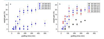
**Figure 2.** Heat induced grafting evaluated by % weight gain for a) different GMA concentrations (% v/v) at 80 °C and b) for 20 and 30% GMA at different polymerization temperatures over a range of polymerization times.
