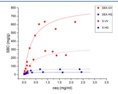
Figure 9. BSA and hIgG adsorption isotherms for UV grafted membranes at 14% weight gain are compared to the adsorption isotherms for heat grafted membranes at 15% weight gain. BSA isotherms are for binding on anion exchange (DEA) membranes, while hIgG isotherms are for binding on cation exchange (S) membranes.
