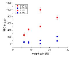
**Figure 5.** Equilibrium protein binding capacity of PBT nonwovens grafted by heat (30% (v/v) GMA, 80  $^{\circ}$ C) and UV light (20% (v/v) GMA) functionalized as anion (DEA) and cation (S) exchangers for capture of BSA and hIgG, respectively.
