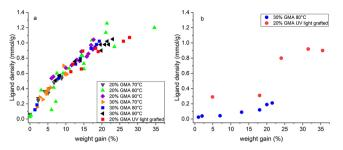
Figure 4. Ligand density of a) DEA and b) Na<sub>2</sub>SO<sub>3</sub> functionalized polyGMA grafted nonwovens.
