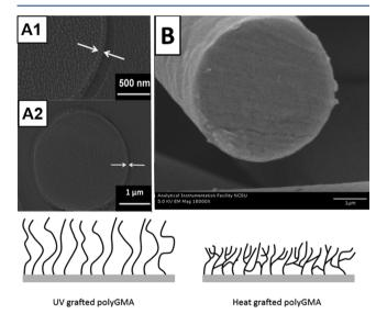
**Figure 6.** SEM images for PBT fiber cross sections grafted with A) UV (A1 and A2 are images with different magnifications of the same fiber)<sup>13</sup> and B) heat induced grafting. Schematic representation of polyGMA grafted layers resulting from UV and heat induced grafting.
