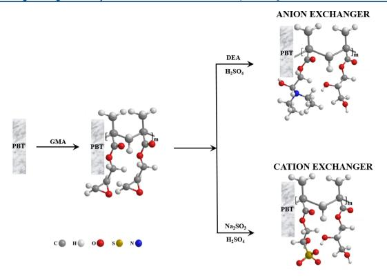
Figure 1. Process of polyGMA grafting and functionalization of PBT nonwovens.
