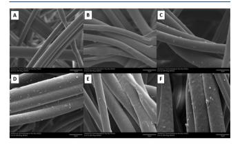
Figure 3. SEM images  $(4,000\times)$  of heat induced grafting onto PBT nonwovens with various % weight gain: A) blank PBT nonwoven, B) 1.5% weight gain, C) 7.5% weight gain, D) 11.5% weight gain, E) 16% weight gain, and F) 19% weight gain.
