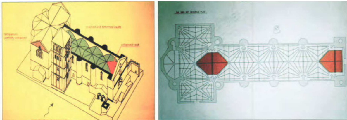
Fig. 19: Damages incurred during the 1997 earthquake in the San Francesco church in Assisi [51].
