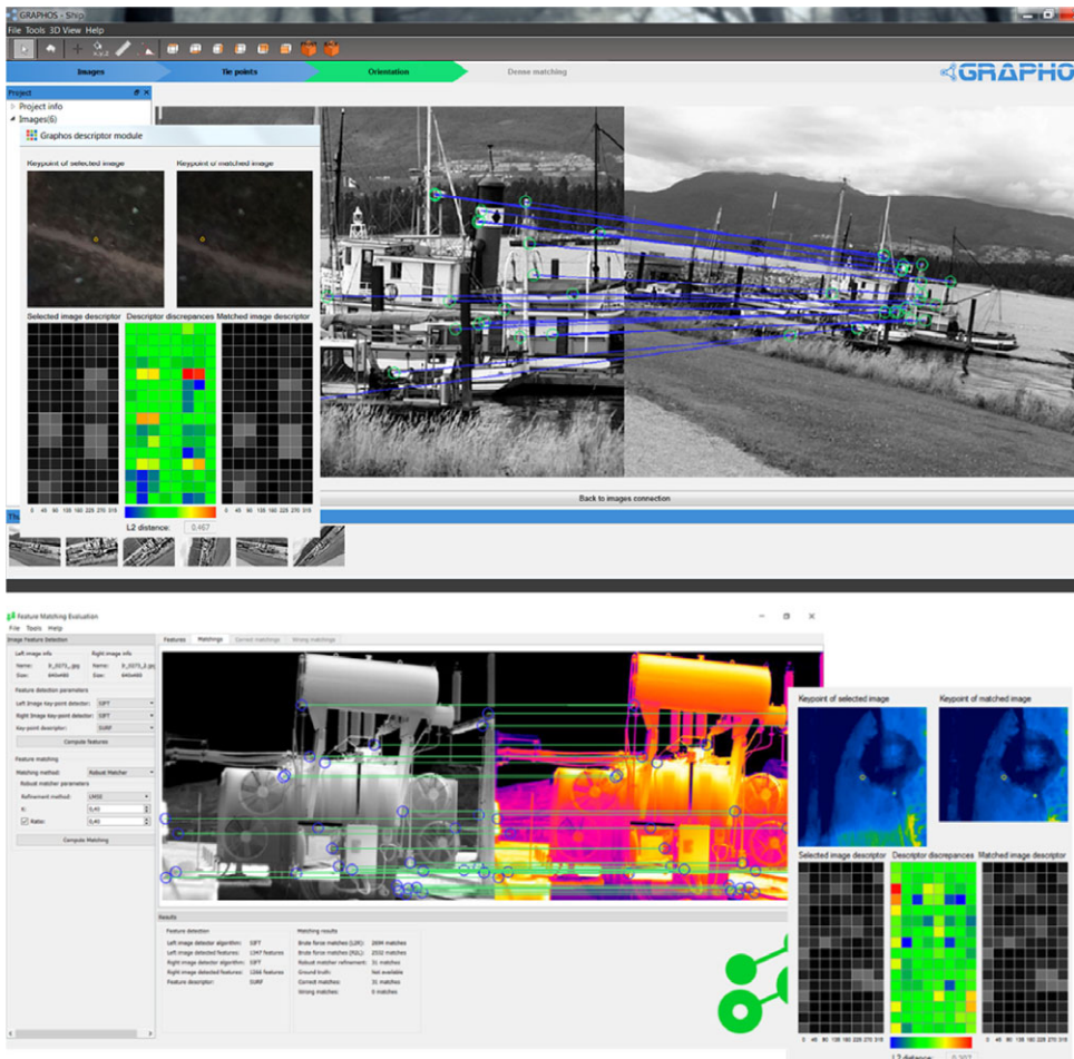
FIG. 3. AMSD feature extraction results on very diverse image scales (top) and among multimodal images (bottom). The graphical representation of the extracted feature points is also shown.
