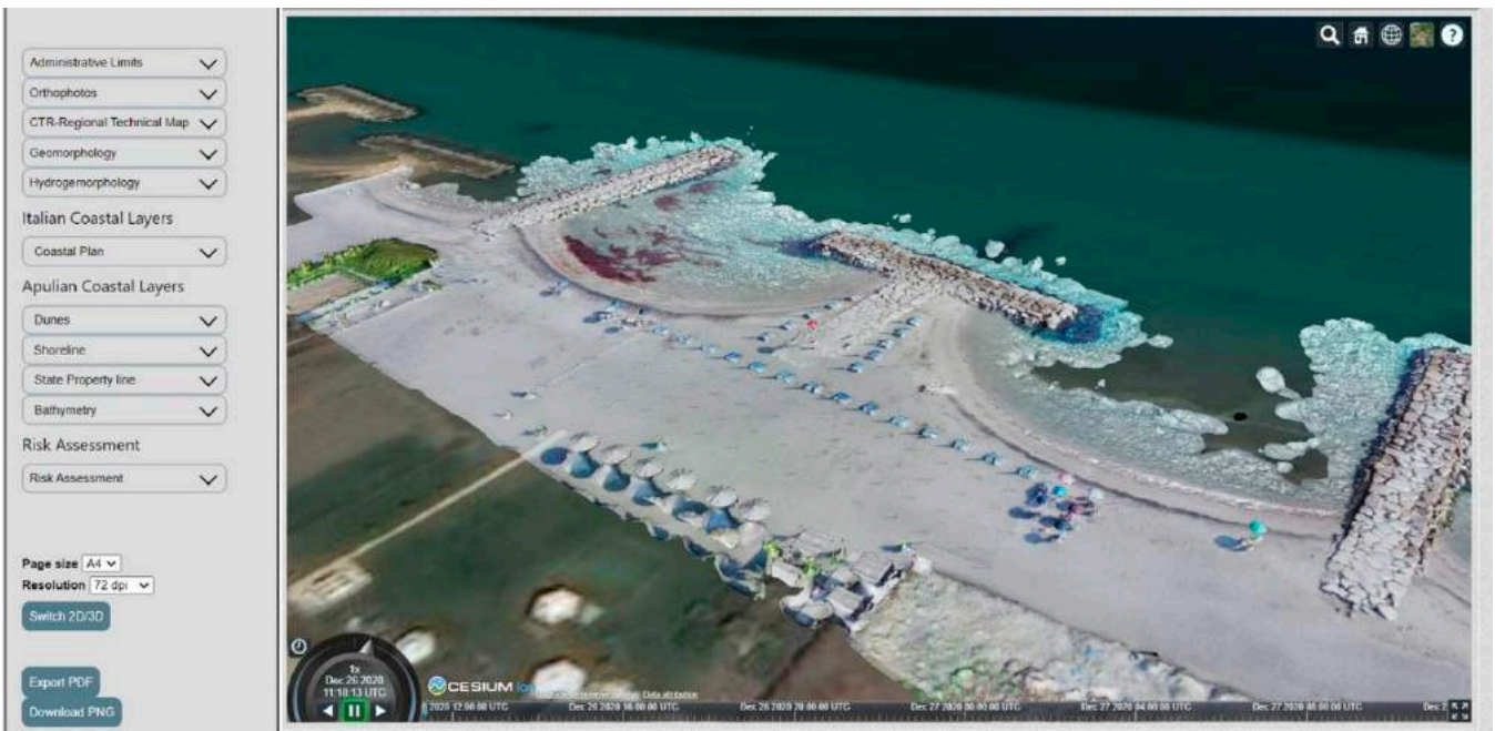
Figure 9. 3D textured mesh extracted by photogrammetric pictures acquired by Remotely Piloted Aircraft Systems (RPAS) of Margherita di Savoia.
