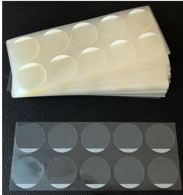
Figure S1. A photo of the sampling discs. D-Squame® brand sampling discs were used in this work.
