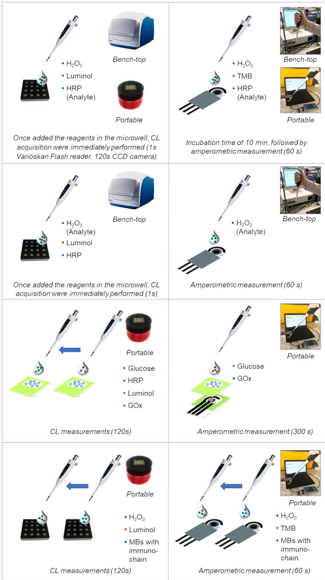
Figure 3. Layout of experimental protocols employed for biosensing measurements in this work.
