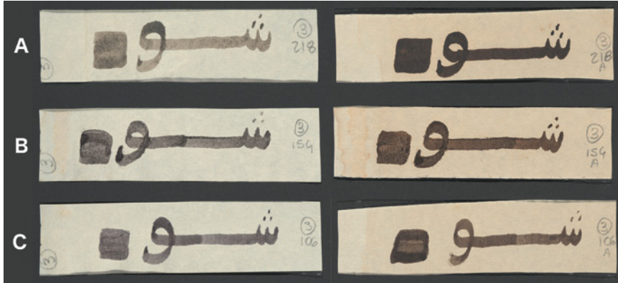
FIGURE 7.5 Samples written with iron gall inks made with iron filings before (on the left) and after (on the right) ageing: A) recipe from contemporary Kenya, ink made with mangrove bark, lemon juice and rusty iron filings; B) recipe by al-Qalalūsi, ink made with bark, vinegar and iron filings; C) recipe by al-Marrākūši, ink made with gall nuts, iron filings and gum arabic
