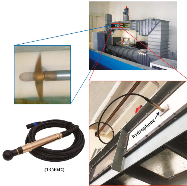
Figure 10. Arrangement of TC4042 hydrophone on cavitation tunnel.
