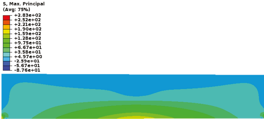
Figure 6. Maximum principal stresses for three-point bending of a simply supported concrete beam.
