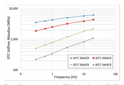
Figure 3. Direct tension-compression (DTC) Isothermal curves for SMACR.
