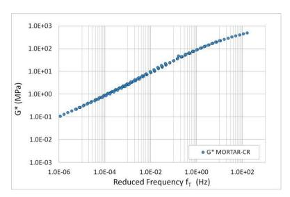
**Figure 6.** MORTAR-CR master curve at 20 °C.
