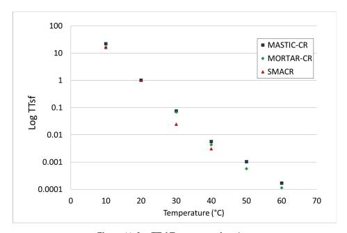
Figure 11. LogTTsf-Temperature function.
