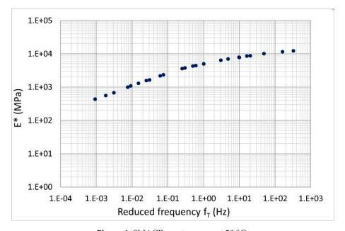
**Figure 4.** SMACR master curve at 20  $^{\circ}$ C.
