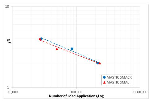
Figure 13. Mastics time sweep test comparison.
