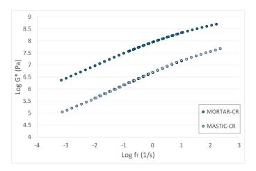
Figure 8. MORTAR-CR and MASTIC-CR master curves.
