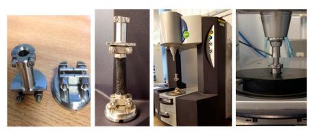
Figure 2. Mortar samples installation and test configuration.
