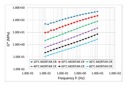
Figure 5. Isothermal curve for MORTAR-CR.
