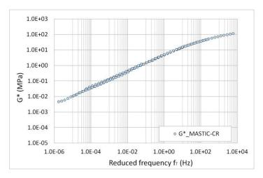
Figure 7. MASTIC-CR master curve at 20 °C.
