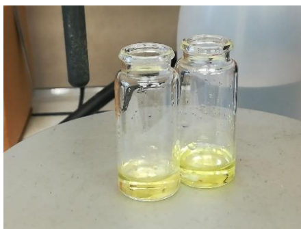
Fig. S3 Fmoc-Tyr(tBu)-OH/DIC/Oxyma Pure=1/1/1 in Sulfolane: Diethyl carbonate=30:70 (left) and Anisole:Dimethyl carbonate=70:30. (right).
