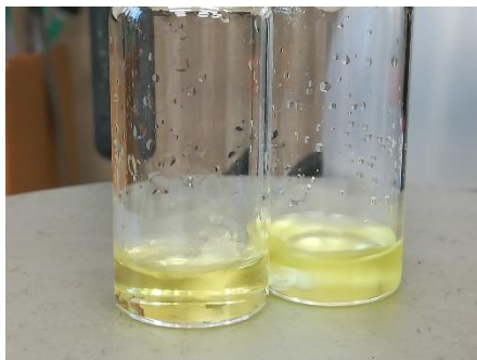
Fig. S2 Fmoc-Leu-OH/DIC/Oxyma Pure=1/1/1 in Sulfolane: Diethyl carbonate=30:70 (left) and Anisole:Dimethyl carbonate=70:30. (right).
