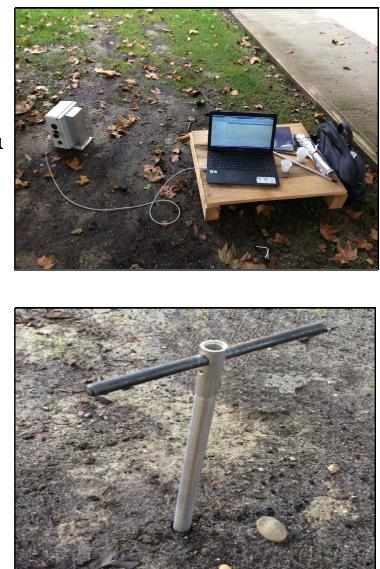
Fig. 4. System acquisition and soil samples coring on real soil.
