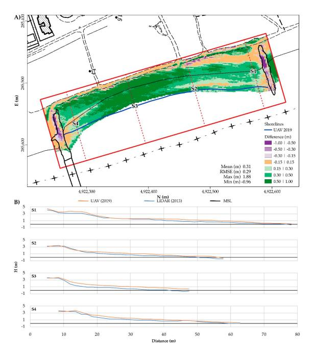
**Figure 8.** Multi-temporal comparison and transect analysis in Lido Adriano area: (**A**) difference between 2019 UAV derived DTM and 2013 LIDAR DTM; (**B**) cross-shore profiles of the beach (S1–S4), 2019 UAV derived DTM (red) and 2013 LIDAR DTM (blue).
