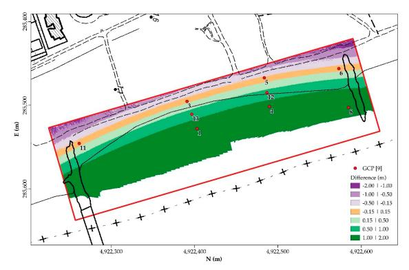
**Figure 4.** The vertical difference in 2019 dataset between the reference survey processed with all 9 GCPs and the test with only 4 aligned GCPs (ID: 11, 3, 5, 6). Axis of rotation highlighted in orange. The Regional Technical Cartography (2013) is shown in black.
