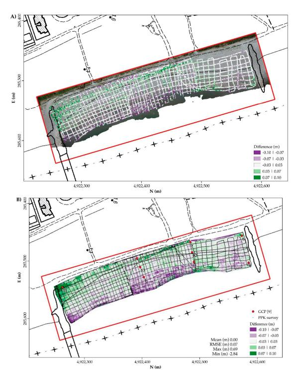
**Figure 6.** Map of the differences between the PPK and photogrammetric DTM. (**A**) height difference over PPK points; (**B**) NRTK assisted- photogrammetric DTMs comparison. The red box highlights the survey area. The GCP location is shown by the red dots.
