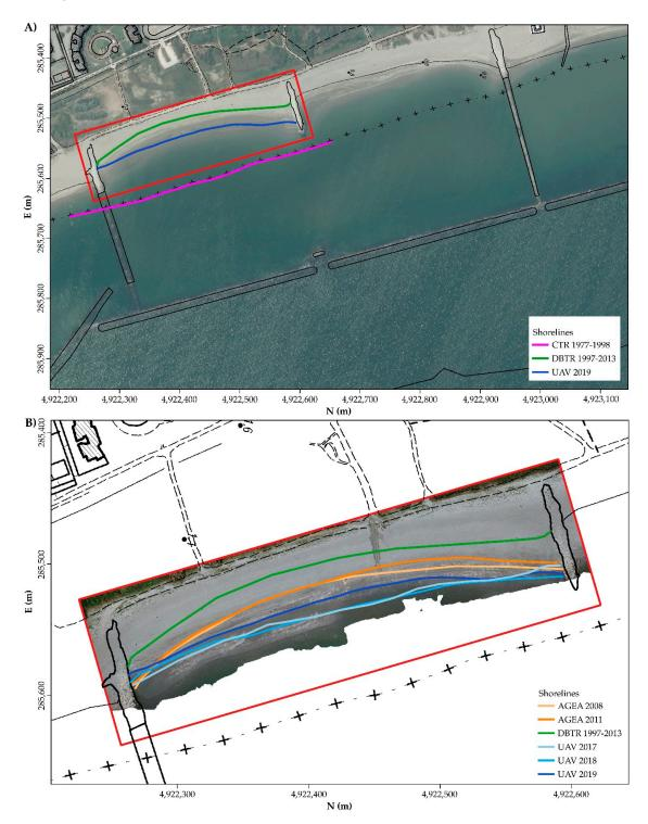
**Figure 7.** Multi-temporal shorelines: (**A**) Key map of the layers Orthophoto AGEA 2011 and DBTR 2013 showing the studied area; (**B**) Detail image of the UAV derived Orthophoto 2019 and the DBTR 2013.
