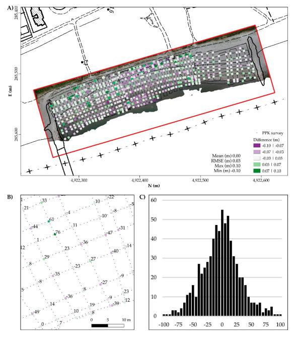
**Figure 5.** Results of the Crossover Error Analysis of track intersections of the 2019 survey. (**A**) map of the 2019 PPK tracks showing the height residuals in different colours, M mean value, RMSE Root Mean Square Error; (**B**) detail of a portion of the surveyed profiles with differences at the crossing points in mm (the same colours of Figure 5A); (**C**) Histogram distribution of the height differences expressed in mm.
