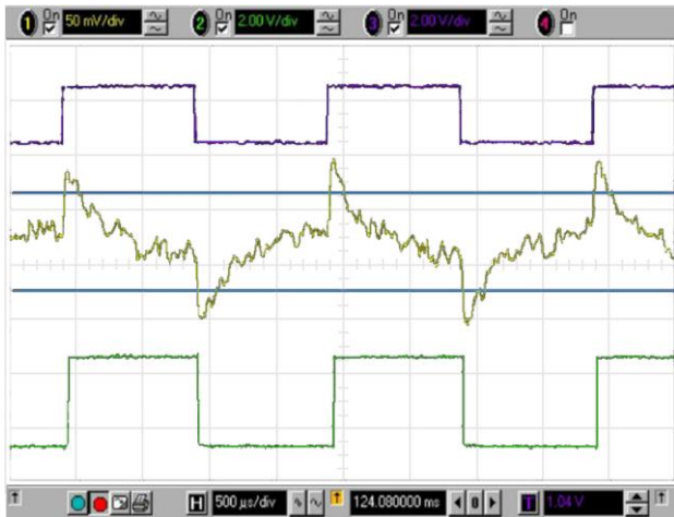
Fig. 20. Measured waveforms corresponding to an input sequence of equal (all 0s or 1s) Manchester-coded bits at 0.5 kbit/s rate. From top to bottom: 1) modulating input signal gating the RF generator; 2) output of the envelope detector; 3) output of the Schmitt trigger. The horizontal blue lines are the trigger thresholds V_H and V_L . RF signal: 771 MHz frequency, -44 dBm amplitude.
