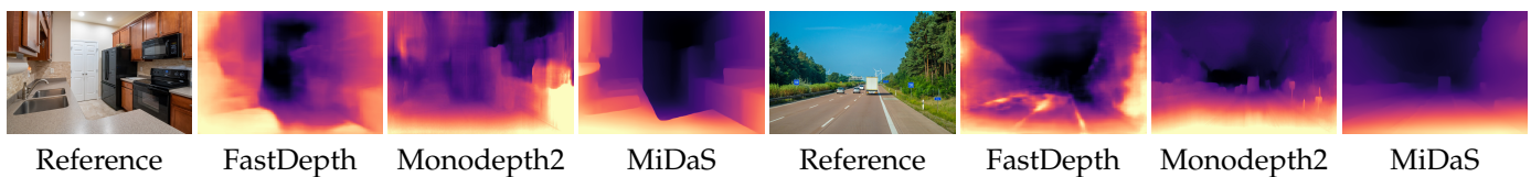
Figure 3. Predictions in the wild. We provide qualitative results for indoor and outdoor Internet images. For each network, we used the checkpoints publicly available. It can be noticed how the networks trained on a single dataset, both in a supervised (FastDepth) and self-supervised (Monodepth2), are not able to generalize well on a different setup. On the contrary, the network trained on various datasets (MiDaS) produced better results. Images from Pexels https://www.pexels.com/ .
