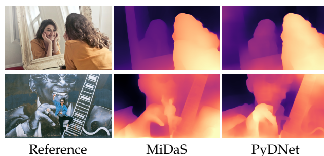
Figure 5. Failure cases. Examples of failure cases of single image depth estimation. From left to right: input image, depth predicted by the teacher and depth predicted by the student.
