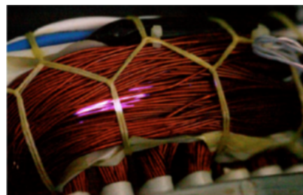
Fig. 1. A typical phase-to-phase insulation failure [4].
