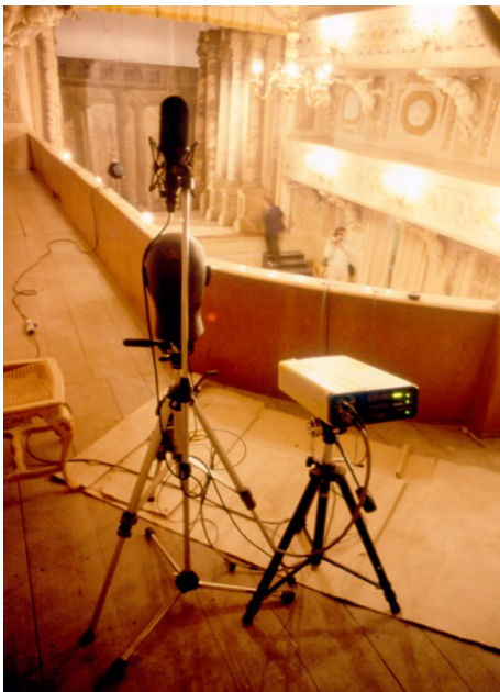
Fig. 3. Instrumentation in the first gallery during the first acoustic campaign.
