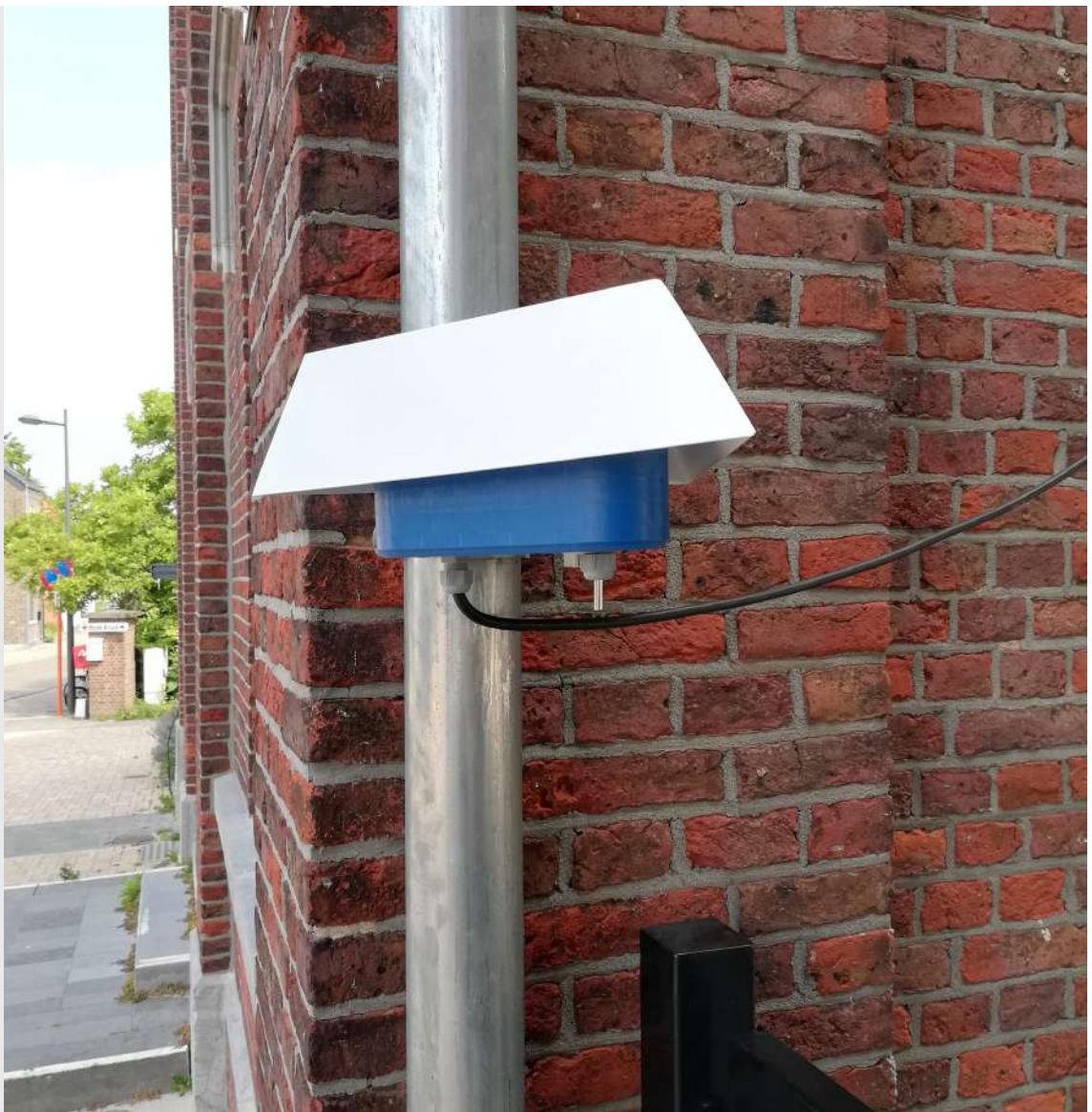
Fig. 14: Deployment of a Living Lab station near the local school to monitor air quality by Hasselt Living Lab, July - September 2019, Hasselt (Belgium)
