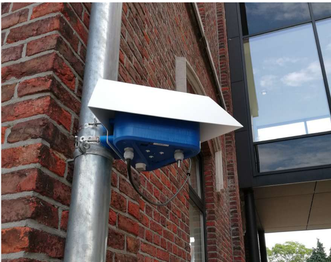
Fig. 28: Deployment of a Living Lab station near the local school to monitor air quality by Hasselt Living Lab, July - September 2019, Hasselt (Belgium)
