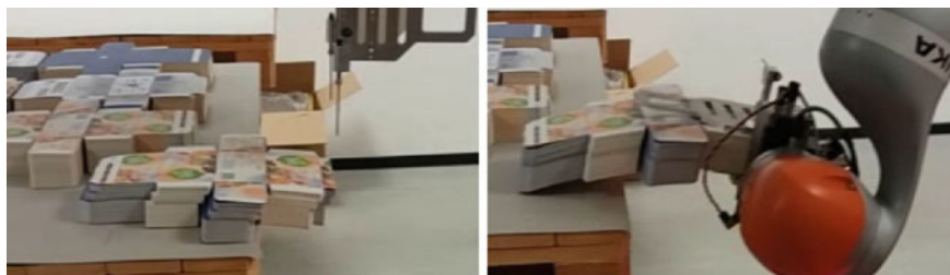
Fig. 7.14 Snapshots of bent blank piles
