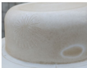
Fig. 3 Lichtenberg figure of the surface charge by using uncharged dust profiles after the spacer was applied with -300 kV inside 0.5 MPa SF_6 for 30 min [15, 29, 30]
