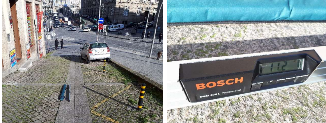
Figure 30: Measuring the slope in a street in Porto (Rua Corpo da Guarda, Porto). Photos by Rui Ramos, CTAC.
