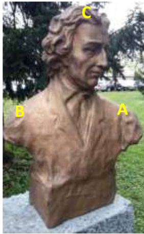
Figure 2: Field test of the bronze statue representing the Slovenian poet France Prešeren in outdoor exposition in the park of ZAG Institute (Slovenia), initially corroded during one year in urban environment. FA-MS coated corroded statue before (left) and after 9 months (right) of natural outdoor exposure.
