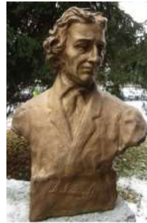
Figure 2: Field test of the bronze statue representing the Slovenian poet France Prešeren in outdoor exposition in the park of ZAG Institute (Slovenia), initially corroded during one year in urban environment. FA-MS coated corroded statue before (left) and after 9 months (right) of natural outdoor exposure.
