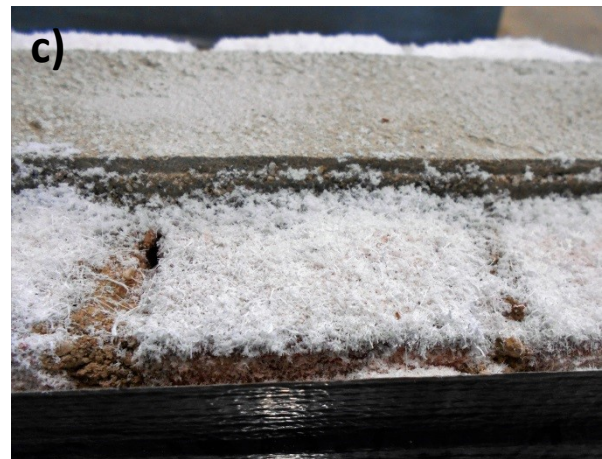
Fig. 6. Photos of selected POST-DRY specimens: a) at the end of the conditioning procedure and after removal of the superficial efflorescence with a metal brush; b) and c) after curing of the composite and before the shear test.
