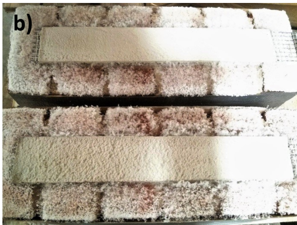
Fig. 6. Photos of selected POST-DRY specimens: a) at the end of the conditioning procedure and after removal of the superficial efflorescence with a metal brush; b) and c) after curing of the composite and before the shear test.
