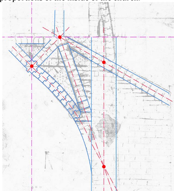
Fig. 4: Axes and intersection points of the load-bearing elements of the lower structure
