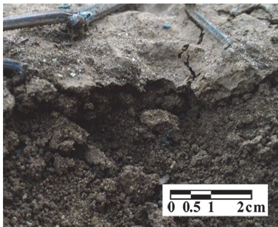
Fig. 2. Surface crust layer developed after the intense storms fallen the 9 th of September 2015, and encountered on the soil surface between the vineyard rows during the second field campaign (see Figure 1). Photo by V. Alagna.
