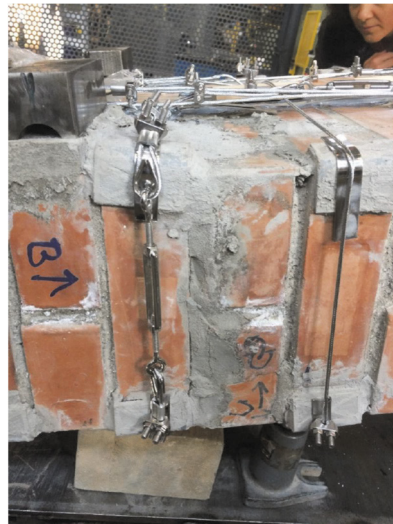
Fig. 13. Mortar/brick disconnection: the stiffness of the longitudinal straps does not allow free rotation around the inner hinge.
