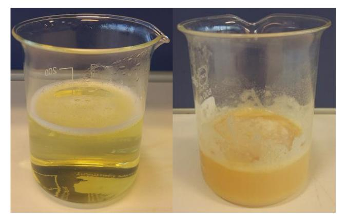
**Figure 2.** (left) Solubilization of ASP in water at 5% w/w in presence of sodium hydrate 0,2 N (pH=8) at 60°C. (right) After cooling, the system appears as a semi-solidified coagel: the dissipation of thermal energy induces the formation of a highly packaged assembling structure.
