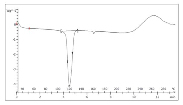
**Graph 3.** Thermogram of ASP. It melts showing an endothermic pick around 115-120°C and an exothermic pick at 260° C.
