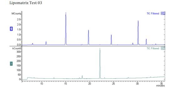
**Graph 4.** GC-MS spectrum of the third aliquot coming from disaggregation test of Lipomatrix in GSF (triplicate analysis).
