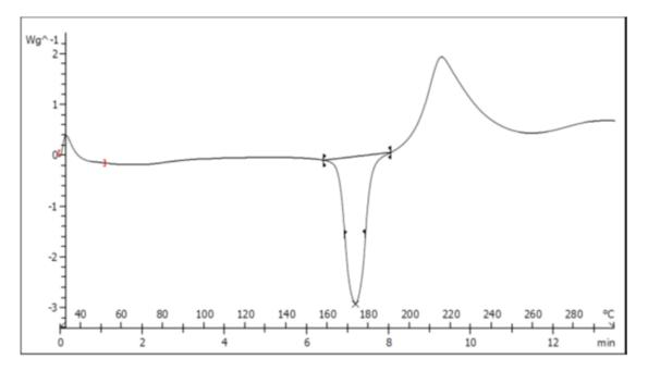
**Graph 6.** Thermogram of Lipomatrix with SRO in the range 30-300°C. It is recognizable a melting phenomenon with an endothermic pick at 170°C, very close to Mannitol one and an exothermic pick between 200 and 240°C.
