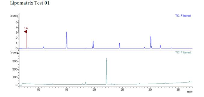
Graph 2. GC-MS spectrum of the first aliquot coming from disaggregation test of Lipomatrix in GSF (triplicate analysis).
