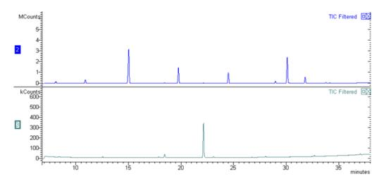
**Graph 3.** GC-MS spectrum of the second aliquot coming from disaggregation test of Lipomatrix in GSF (triplicate analysis).
