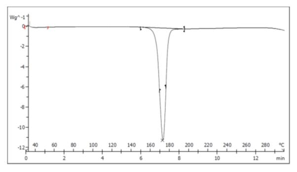
**Graph 2.** Thermogram of Mannitol. it shows an endothermic fusion pick at 170°C, data according to the technical data sheet of the raw material for melting point.
