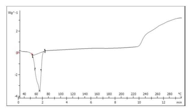
Graph 1. Thermogram of MDGFA. It is recognizable an endothermic melting pick between
