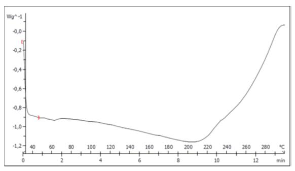
**Graph 4.** Thermogram of SRO (30-300°C). The thermogram shows an exothermic large pick after 210°C, likely corresponding to the oil degradation; it was not possible to investigate the typical exothermic crystallization behavior of a vegetable oil, because the device employed was not equipped with an intracooler.
