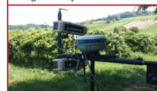
Fig. 2. GreenSeeker® sensors used to acquire NDVI.
