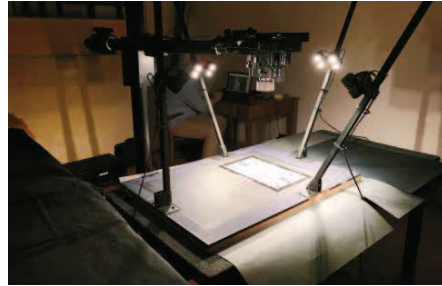
Fig. 4. The solution for the structure to support the lighting system and hold the drawing, with the column holding the Rencay DiRECT Camera Systems 24k 3 (digital scan back and camera) in position at the Gabinetto Disegni e Stampe, Uffizi Gallery.
