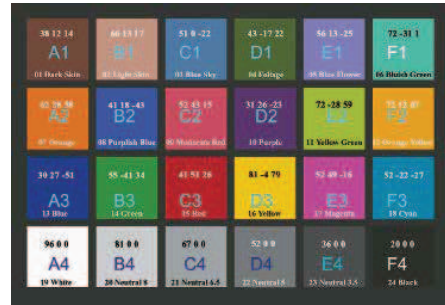
Fig. 12. The X-Rite Color Checker (CC) Classic targets with CIEXYZ colour values and their identification.
