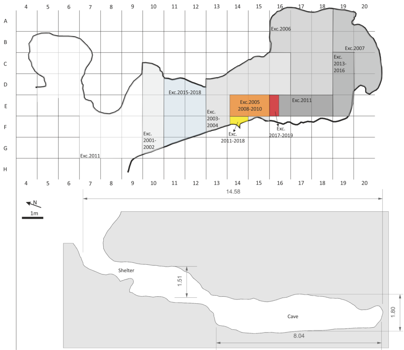
Figure 5: Planimetry of the cave (modified after Pennacchioni) showing the excavated areas. Longitudinal section of the cave obtained by ortho-photo of the cave produced by 3D laser scanning (drawing L. Repola).
