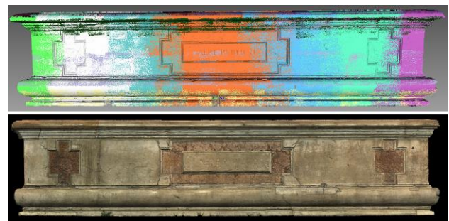
Figure 11. East side of the basement; the numerous scans acquired (top); the complete photo-textured mesh (bottom).
