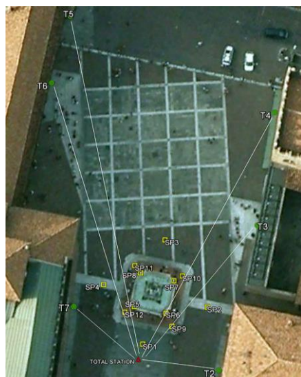
Figure 4. The scan positions of the laser scanner survey (yellow squares) and the targets used for the definition of the reference system (green circles).
