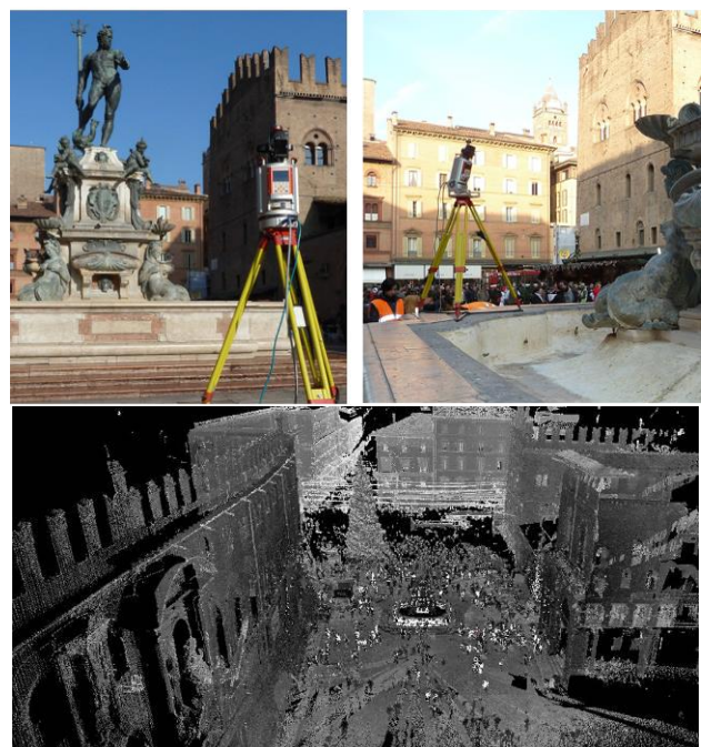
Figure 2. Two moments of the laser scanning survey (top); one of the acquired point cloud (bottom).
