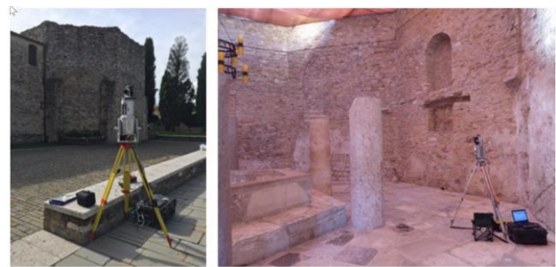
Figure 2. Acquisition of outside (left) and inside (right) using TLS
