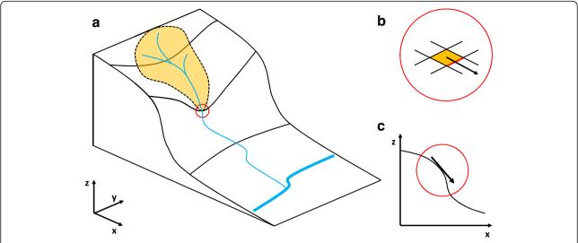
Fig. 1 TWI scheme Scheme of the TWI: a Flow accumulation area, b Flow direction and the corresponding flow width for a DEM cell, c Tangent of the slope angle
